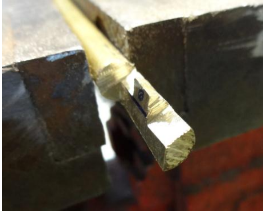
Figure 9: Here the two sections marked 45° have been filed. The center section, Marked 0° remains untouched.
