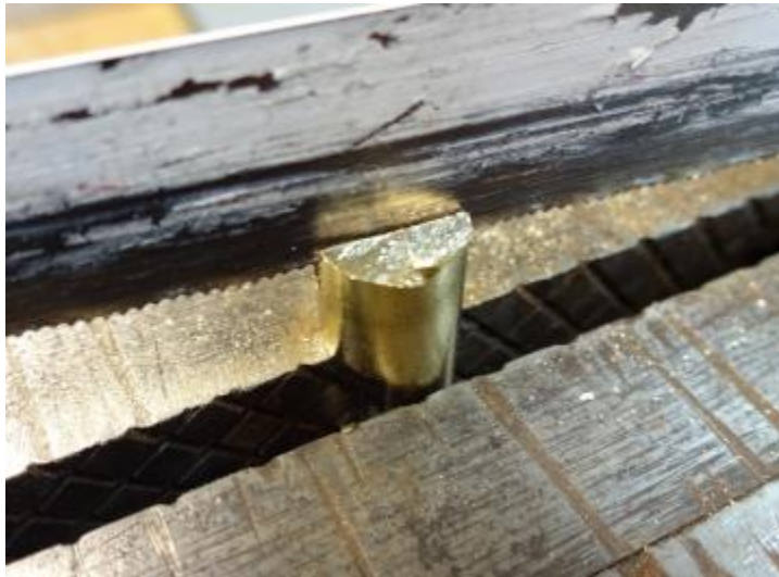
Figure 10: In the top of the key use a hacksaw to cut a slot for the bow (the washer). Knock off the sharp edges on a wire wheel or with a hand file.
