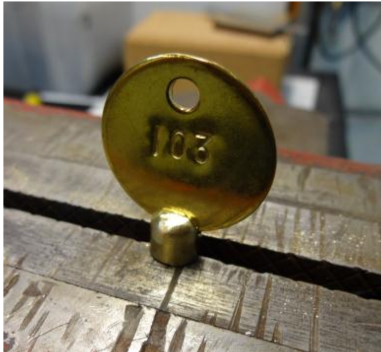
Figure 12: Next I tap the bow into the slot. You can either epoxy it in place or silver solder it. I prefer to silver solder it because it'll last longer.
