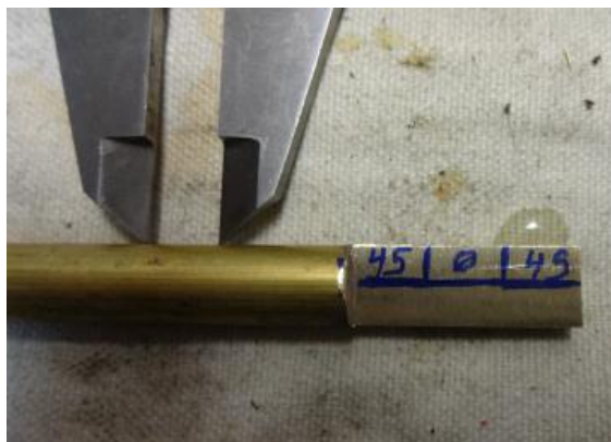
Figure 8: Next, refer to the bitting chart and mark off the three bits. Each bit is 0.30" wide. In this case, I am making a key for a number 103 lock I bought on eBay for $21.
