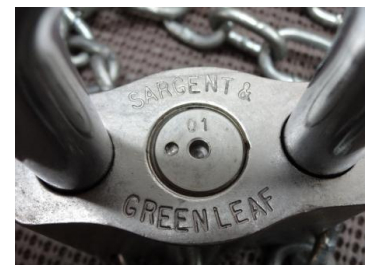
Figure 4: Key number marking on top of lock
