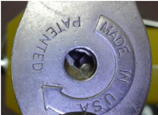
Figure 5: You can see the three "half-moon" shaped disks in the key hole.
