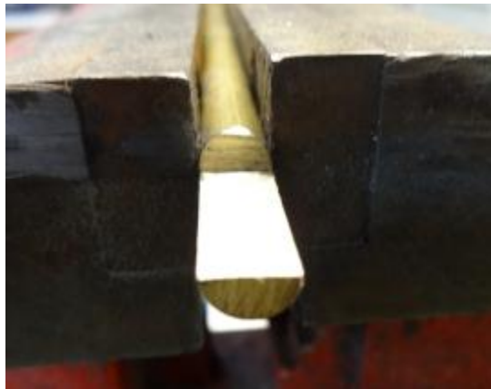
Figure 7: File it until you have a half-round profile that is 0.90" long. This is your blank key.
